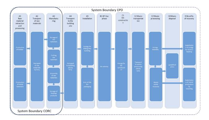
Figure 1: Flowchart for Roof truss production
